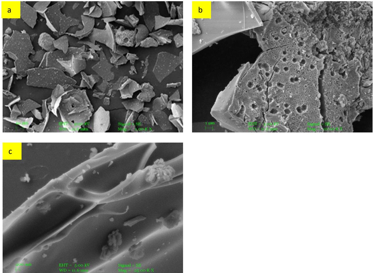
Fig 3. SEM analysed structural morphology of silicate (a) Platy structure, (b) Porous Structure, (c) Magnified view of a platy structure
